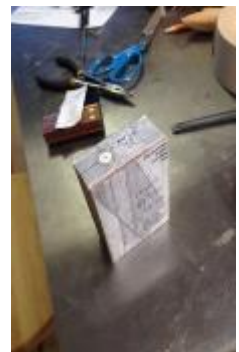
Figure 2. Pattern on wood PHJ blank
