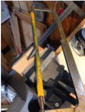
Figure 6. Cut pipe to wood as close as possible.
