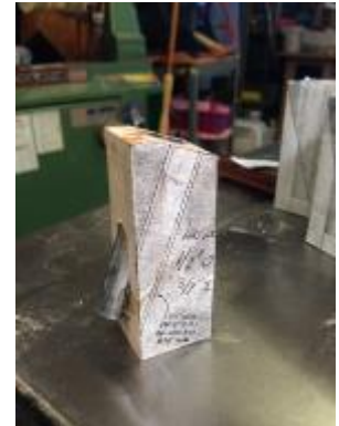
Figure 5. Pipe epoxyed in wood blank.
